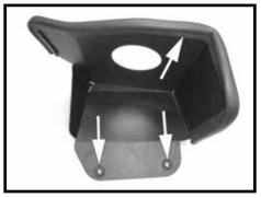
Step 11 Install the rubber bulb seal, this may require trimming to the correct length. Install the grommet removed from Step 10.
