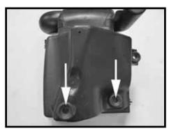
Step 10 Remove the factory grommets from the air box. They will be reused on the next step.
